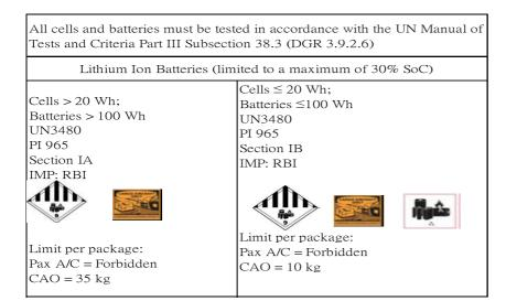
UN38.3 Lithium ion cells and batteries have been successfully testing and comply with the UN Model Regulations, Manual of Test and Criteria, Part III, subsection 38.3
